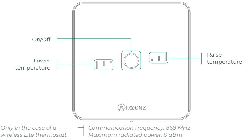
**Note:** To access the Lite settings parameter, from any Airzone Blueface thermostat you must access the zone controlled by your Lite thermostat using the Zone navigation option. (See Zone settings section).
