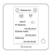
For the correct identification at the BACnet/IP network and the correct functioning of the Airzone BACnet Interface, it may be necessary the modification of the following configuration parameters:
