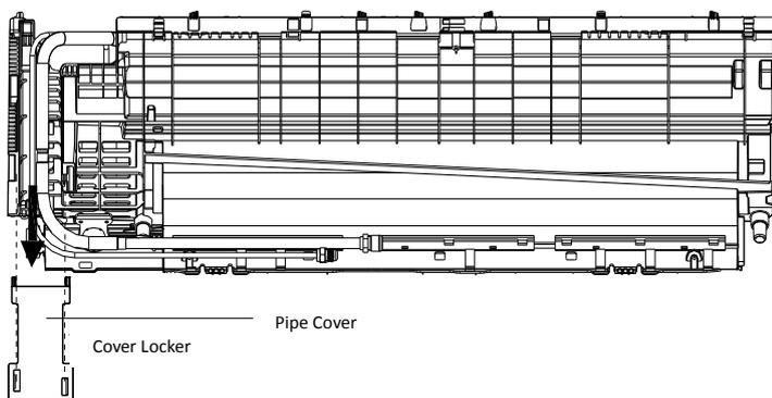
9. Disassembly the evaporator
