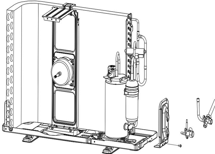
**step9: Disassemble the 4-way valve assembly**
