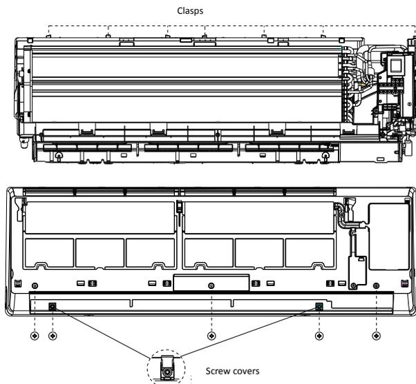
7. Disassembly the electric control box.
