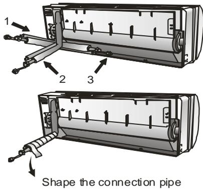
When extending the drain hose at the indoor unit, install the drain pipe.
