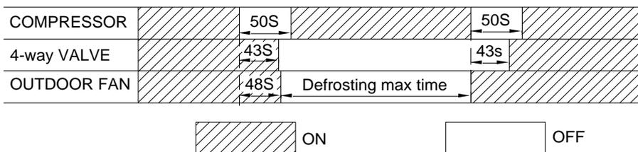
**Defrosting end off:** Compressor stops working, and re-starts to working after 50s delay;
