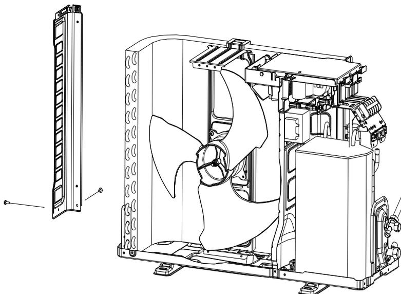
**step4: Disassemble the Axis Fan Blade**
