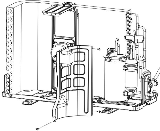
**step8: Disassemble the 2 and 3-way valve**
