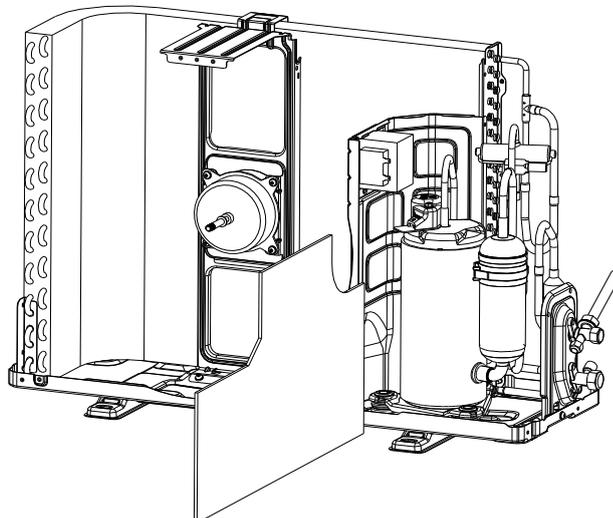
**step7: Disassemble the separate plate**
