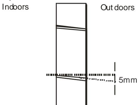
The hole must slope downwards towards the exterior.
