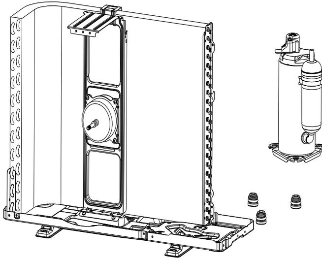
**step11: Remove the fan motor and fan supporter.**
