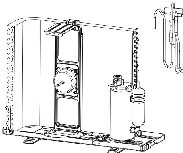
**step10: Disassemble the compressor.**
