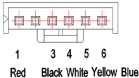
**2. Outdoor DC Fan Motor (control chip is in outdoor PCB)**
