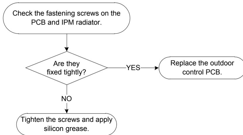
**Note:** For certain models, outdoor PCB could not be removed separately. In this case, the outdoor electric control box should be replaced as a whole.
