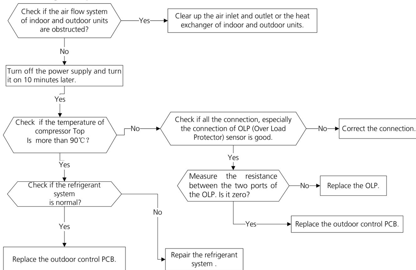
**Note:** For certain models, outdoor PCB could not be removed separately. In this case, the outdoor electric control box should be replaced as a whole.
