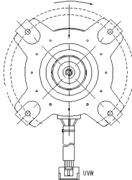
**2. DC Fan Motor(control chip is in fan motor, single fan)**
