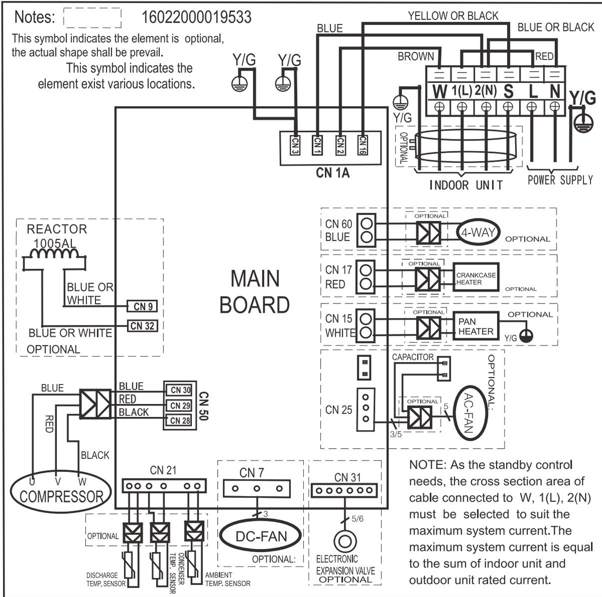
Outdoor unit wiring diagram: 16022000B 13817
