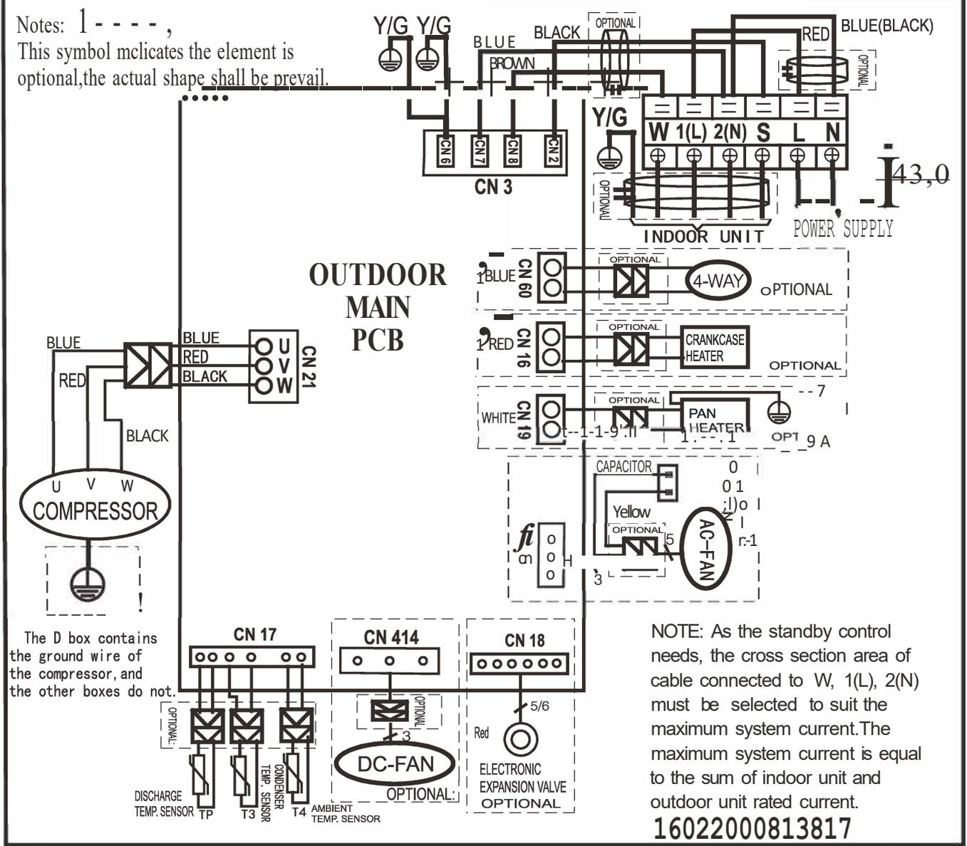
Outdoor unit printed circuit board diagram: 17122000044714, 17122000048121, 17122000046453
