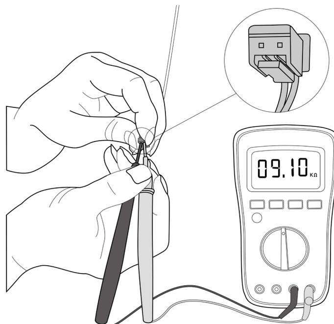
**Note:** For certain models, outdoor PCB could not be removed separately. In this case, the outdoor electric control box should be replaced as a whole. For certain models, outdoor unit uses combination sensor, T3,T4 and TP are the same of sensor. This picture and the value are only for reference, actual appearance and value may vary.
