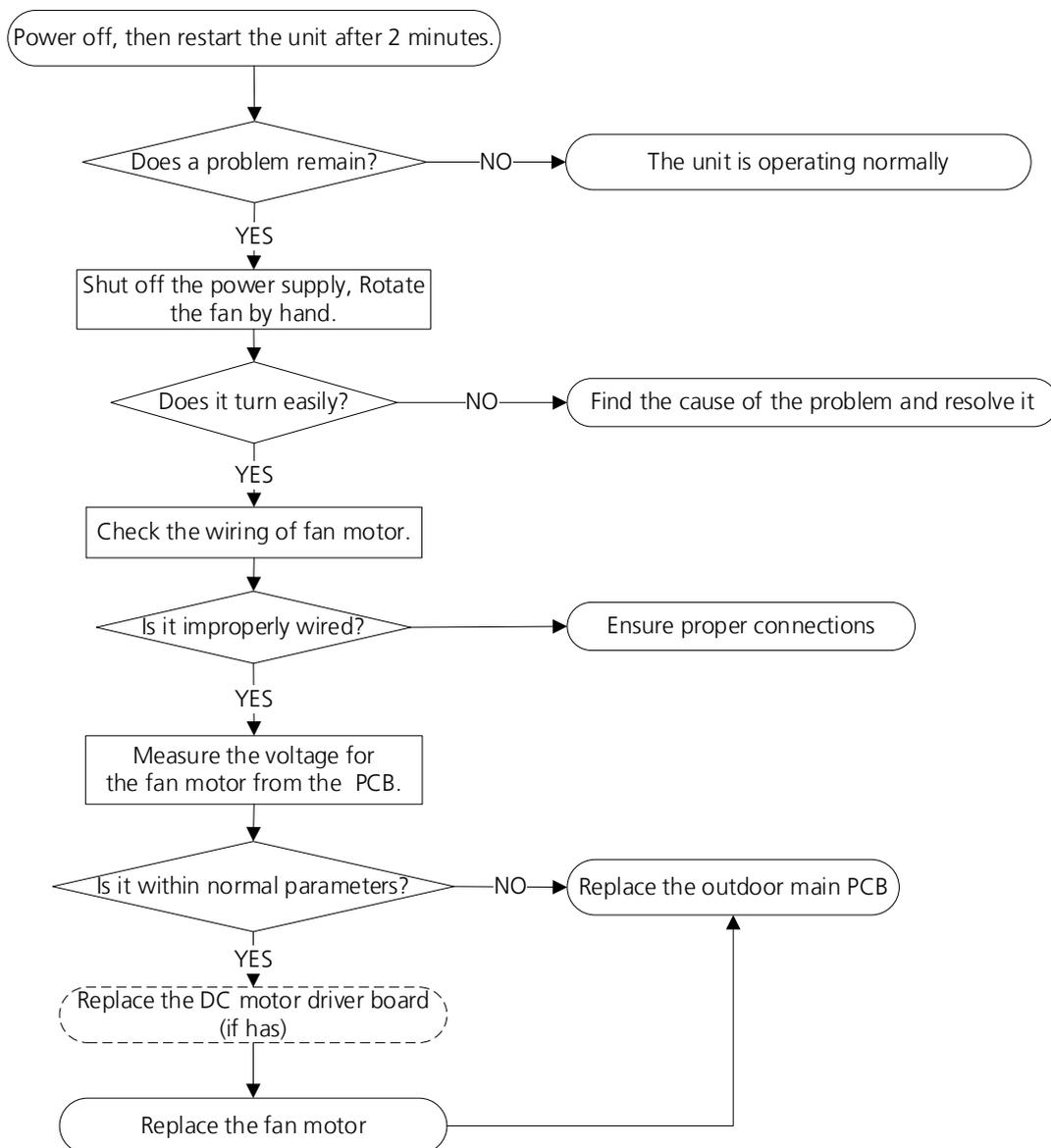
**Note:** For certain models, outdoor PCB could not be removed separately. In this case, the outdoor electric control box should be replaced as a whole.
