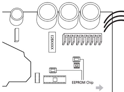
**Note:** For certain models, outdoor PCB could not be removed separately. In this case, the outdoor electric control box should be replaced as a whole. This pictures are only for reference, actual appearance may vary.
