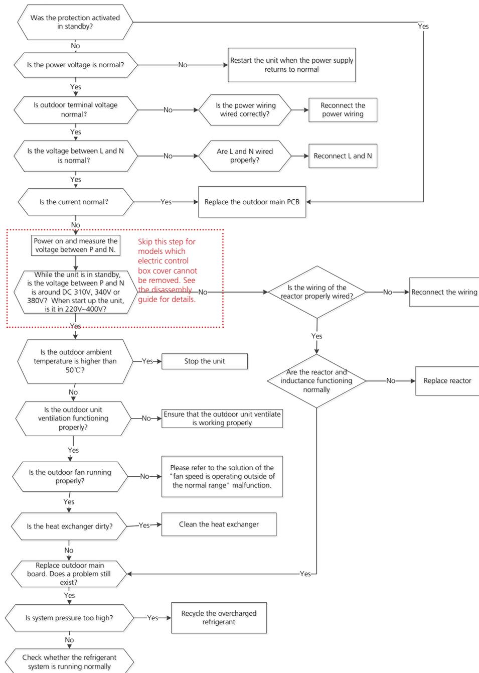
**Note:** For certain models, outdoor PCB could not be removed separately. In this case, the outdoor electric control box should be replaced as a whole.
